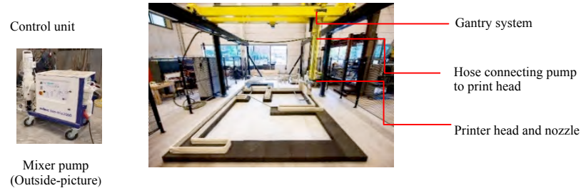
Figure 1. 3D printing facility at TU/e, with some examples of printed objects.
