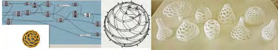
Figure 1. Parametric model of the reconfigured pinecone and 3d-printed family of forms.
