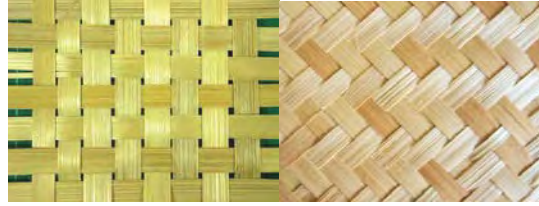
Figure 5. Single and double pattern of biaxial woven patterns.
