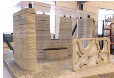
Figure 3. 3D concrete printed pavilion
