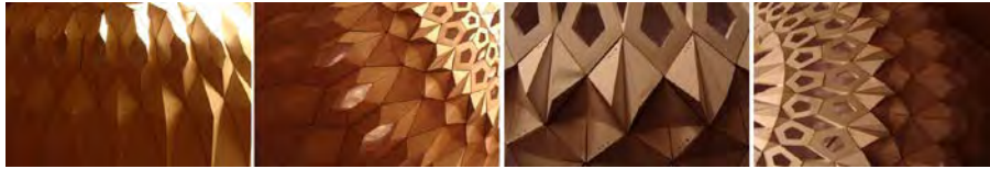
Figure 3. Digital Karbandi; final mock-up made with flat but folded pieces
