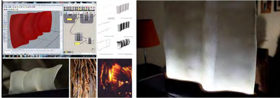
Figure 5. Kangaroo model of surface, 3d printed model and natural formations
