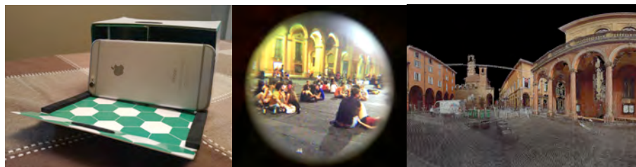
Figure 2. The 3D point cloud, visualized into a cheap, immersive environment using a simple smartphone.
