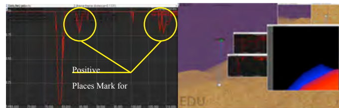
Figures 4 & 5. Correct ground registration via ray and vision sensors.
