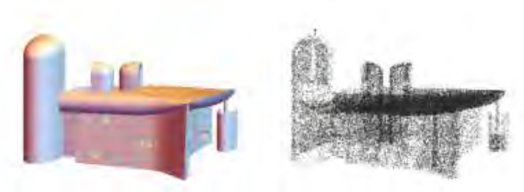
Figure 2. (a) 3D region as continuous domain in Euclidean space, (b) vector quantization of the region. The 3D region must be modeled as an error-free closed three-dimensional mesh.
