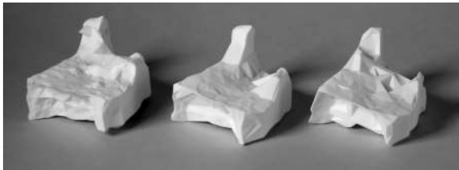
Figure 4. Printed meshes on Le Corbusier's chapel generated by \alpha -shapes from one, two and three-dimensional array SOMs (from left to right).
