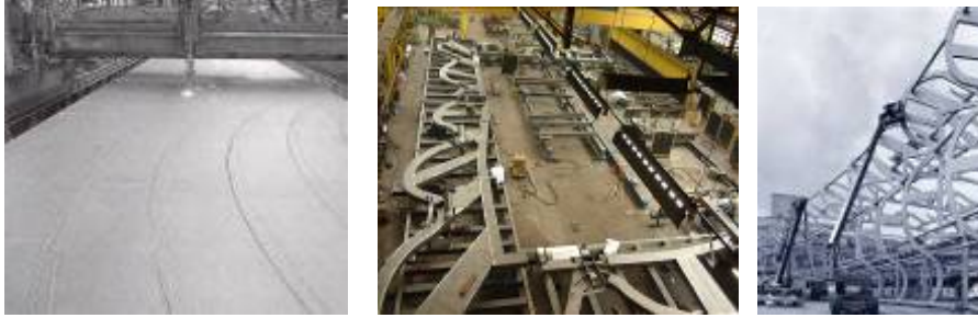
Figure 5 CNC plasma cutting of steel sheet, Welding, fabrication of the hollow box steel girders, Assembly of the steel structure of Dynaform, 2002, Frankfurt am Main, Germany Source: http://www.gregull-spang.de/content/Referenzen-Bilder-Messehallen-BMW.htm
