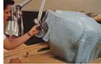
Figure 4 Model being digitized by 3D scanner, EMPproject, 1995-2000
