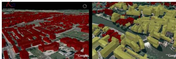
Figure 1. City of Bamberg in Google Earth: Structure model with ca. 50000 buildings; higher level of detail with roof structures
