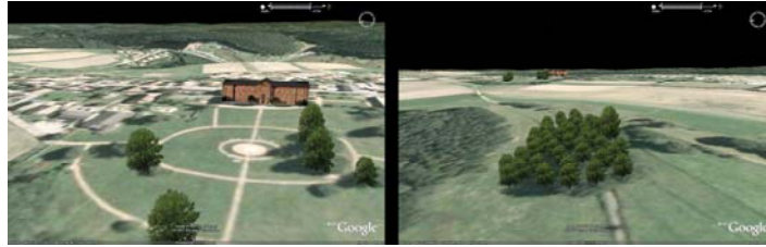
Figure 5. Textured model of Trippstadt castle; Integration of a wood area, by using linked textures, the file size for one tree is as small as for 1000 trees
