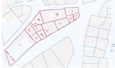
Figure 3. Example of a map where surveyors have outlined and numbered some buildings.
