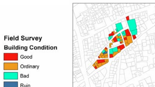
Figure 5. Building condition map showing many building in bad condition (cyan) and a single ruin (blue).
