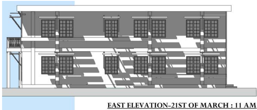
Figure 5. Simulation of Shading Devices as add-ons to the façade, elevation; Maha Aljarrah, Spring 2007
