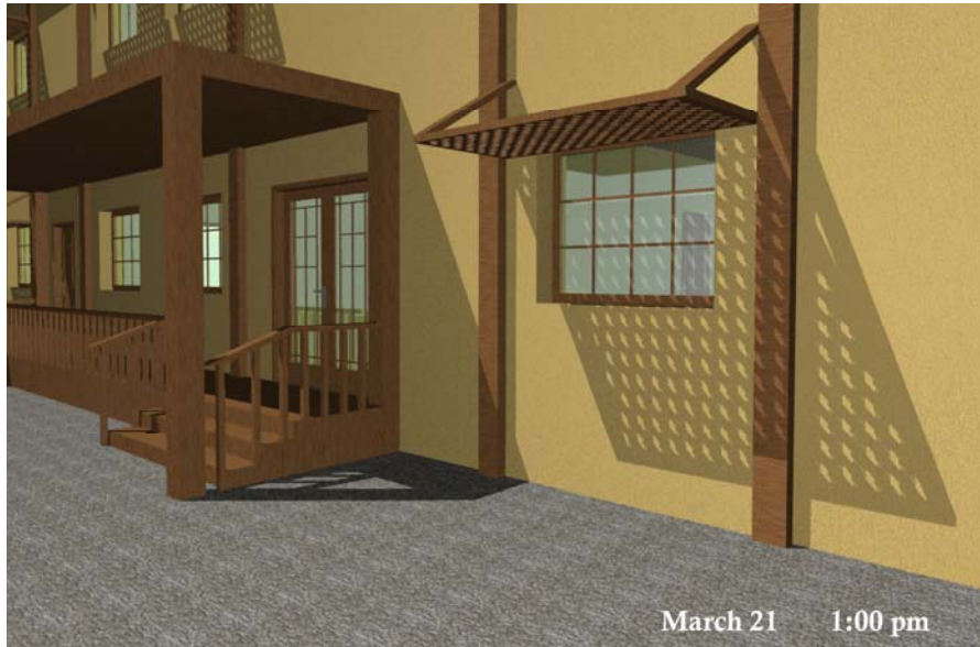
Figure 7. Simulation of Shading Devices as add-ons to the façade, perspective; Meera Al-Qassimi, Spring 2007
