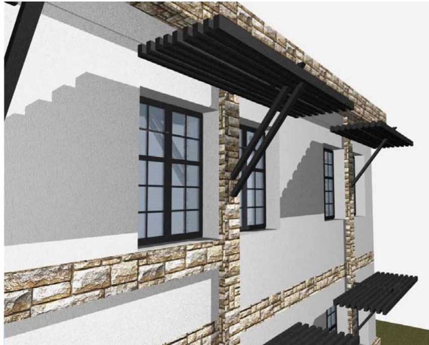
Figure 6. Simulation of Shading Devices as add-ons to the façade, perspective; Maha Aljarrah, Spring 2007
