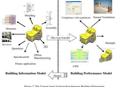
Figure 2: The Current level of integration between Building Information Modelling and Building Performance Modelling. \* Note that this is a one way transfer of the 3D model and has only been achieved by only one company.
