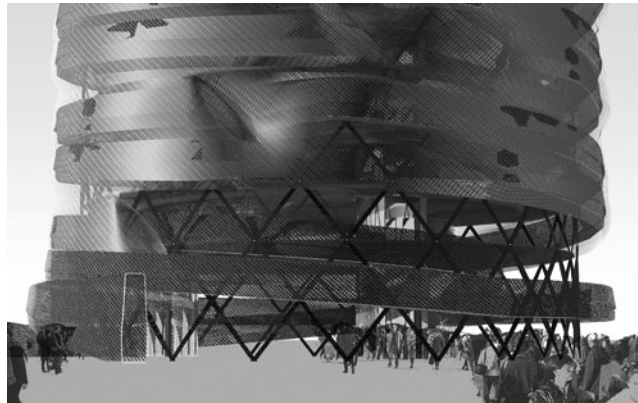
Figure 4. Carbon Tower (Peter Testa) – Using a software called Weaver , this building’s external envelope is woven rigid from ultra-light composite metals. The result is a building whose surface is simultaneously a self-contained support. Source: http://archrecord.construction.com/innovation/2_Features/0310carbonfiber.asp
