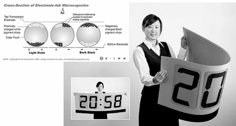
Figure 5. Bendable Clock (Citizen) – This unique design is enabled by E Ink(r)Imaging Film. Architecture is yet to exploit such new surface technologies. See www.eink.com
