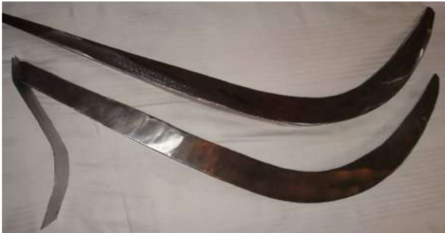
Figure 7. Scaled models of a column of Brasilia's Cathedral. The top one was digitally fabricated and the bottom one was analogically produced.
